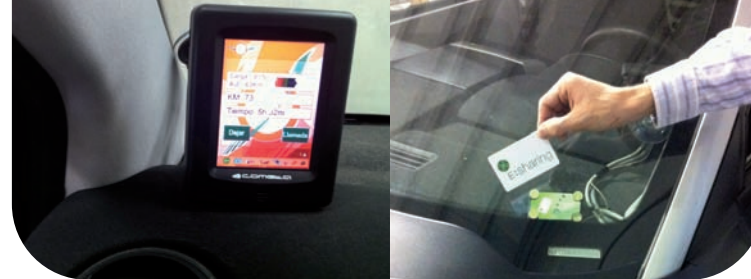
Electric vehicle reader (on the left) and starting card
